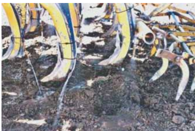
FIGURE 5.11 Spray lines attached behind each planting tyne/boot dispense inoculants by water injection.
