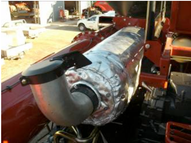
Fig 6. An aftermarket insulating shield or muff on a Case AFX header that encloses the exhaust pipe and turbocharger, similar to units used in marine applications. (Product Source: COLPRO, Pendle Hill ,NSW. www.colpro.com.au )
