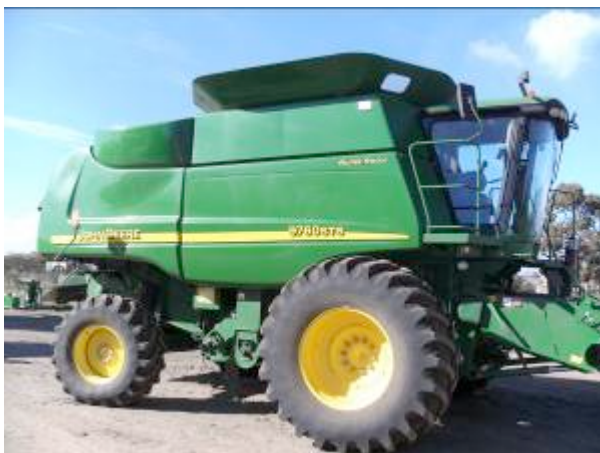
Fig 8. On the latest 70 series STS models, Deere have relocated the inlet to the rad fan. This forces cooling air to come in from atop the machine instead of where it used to be on the RHS.
