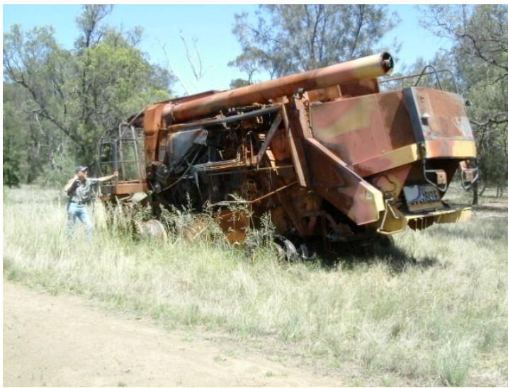
Figs 1, 2. Combine Harvester fires afflict all brands. Right: The heat from this fire in an 8020 harvesting chick peas was so intense that both axles sagged and bent out of shape.
