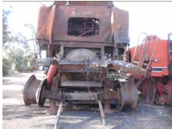
Figs 1, 2. Combine Harvester fires afflict all brands. Right: The heat from this fire in an 8020 harvesting chick peas was so intense that both axles sagged and bent out of shape.
