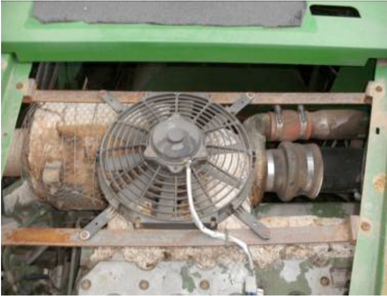
Fig 9. Engine bay modifications. This is a farmer-installed extra fan (ex-Auto) and insulation wrapping around the exhaust system on an STS by Custom Contractor Harry Roper in Goondiwindi. The non-standard shield wrapped around the exhaust system has not caused any turbo problems so far but it is not a Company authorized fitment.
