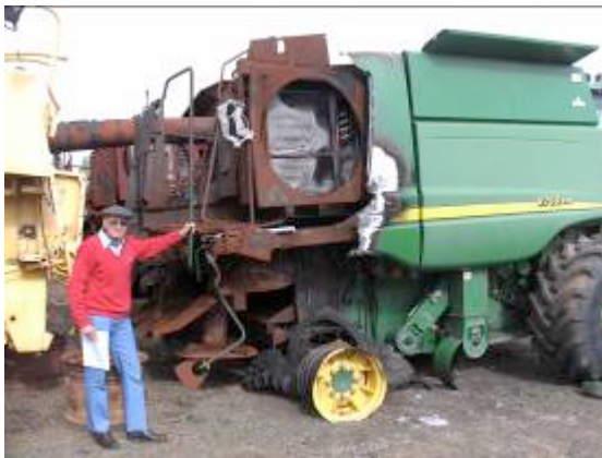
Figs 1, 2. Combine Harvester fires afflict all brands. Right: The heat from this fire in an 8020 harvesting chick peas was so intense that both axles sagged and bent out of shape.
