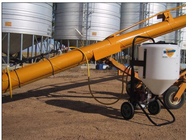
Peat inoculum can be applied with a low pressure applicator. The auger mixes the inoculant with the seed. Courtesy of Peter Munns from Time Saver Industries.
